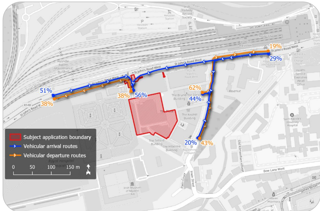
Figure 10 – HSQ vehicular trip origin/destination proportions – AM peak (map data & imagery: OSM Contributors)
